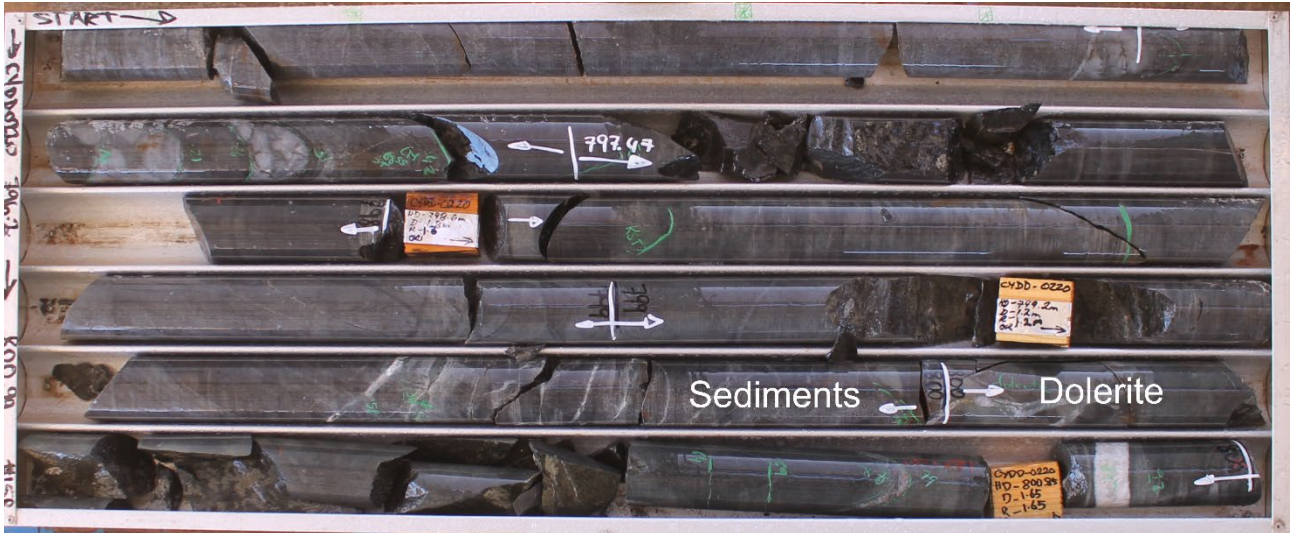
Figure 6: Photo of drill core from CYDD0220 from 796.2m to 800.99m down hole. Upper contact between sediments and poorly tested Dolerite. Note assays are not available for this hole – assumed to have been returned after the operation went on care and maintenance and then lost.
