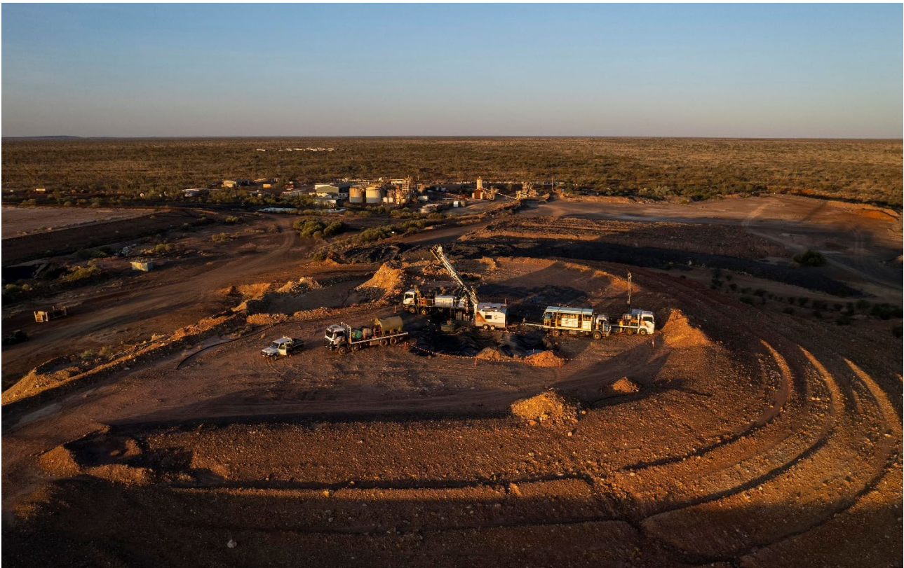
Figure 1: Diamond drilling to extend and upgrade the Kavanagh Resource with ROM stockpiles, processing facility and camp in the background
