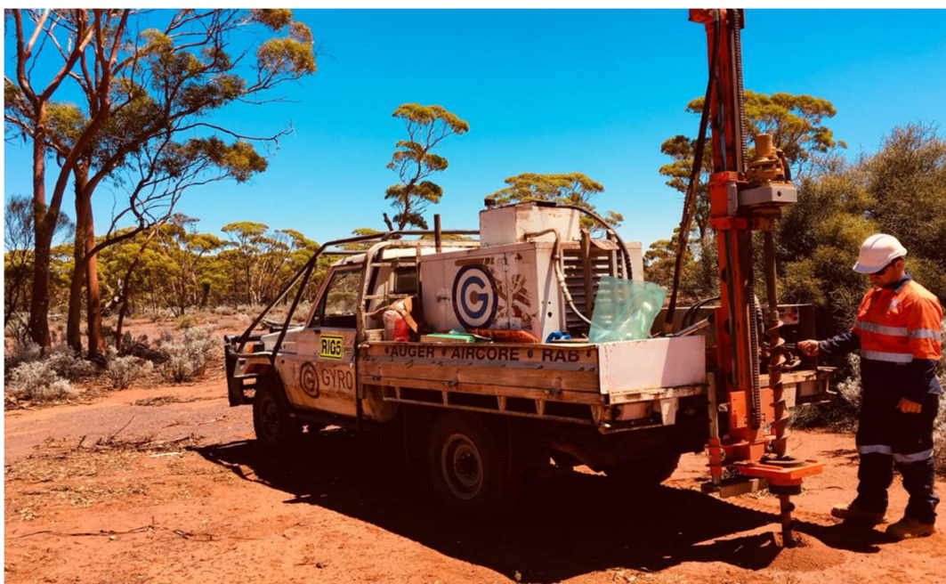
Figure 1: Auger drilling at Balagundi, part of the Kal East Gold Project
