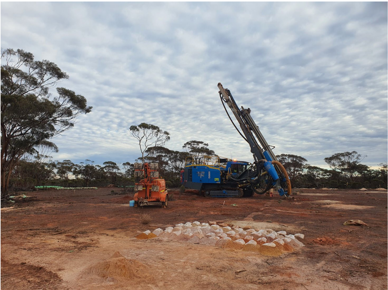
Figure 1: Rig and ancillary equipment on site at Myhree to complete grade control of the Ore Reserve.
