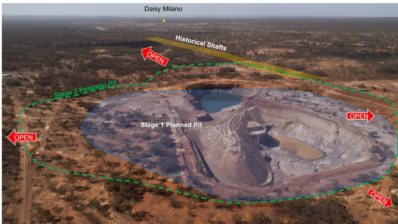
Figure 1. Aerial view of Fingals Fortune area looking south with potential pit outlines and ~750m long trend containing pre-WW1 shafts
