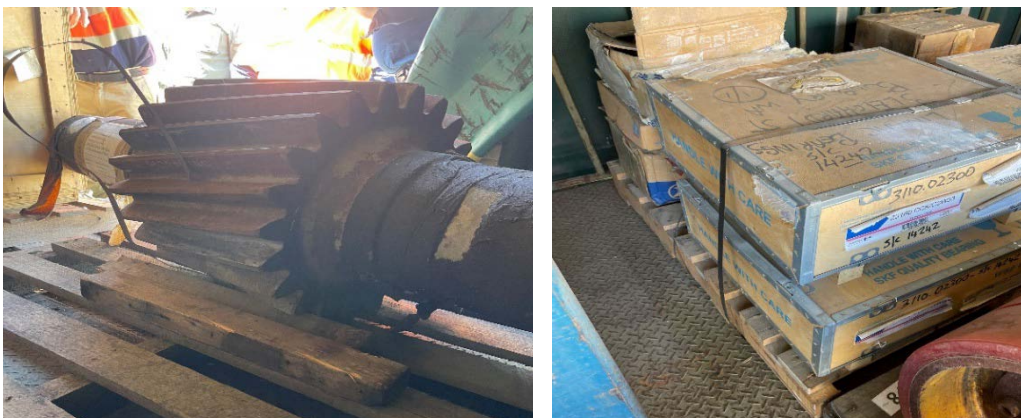
Figure 4: The Option includes numerous critical spares including pinions (left) and brand-new bearings (right). All spares are well stored and in good condition.
