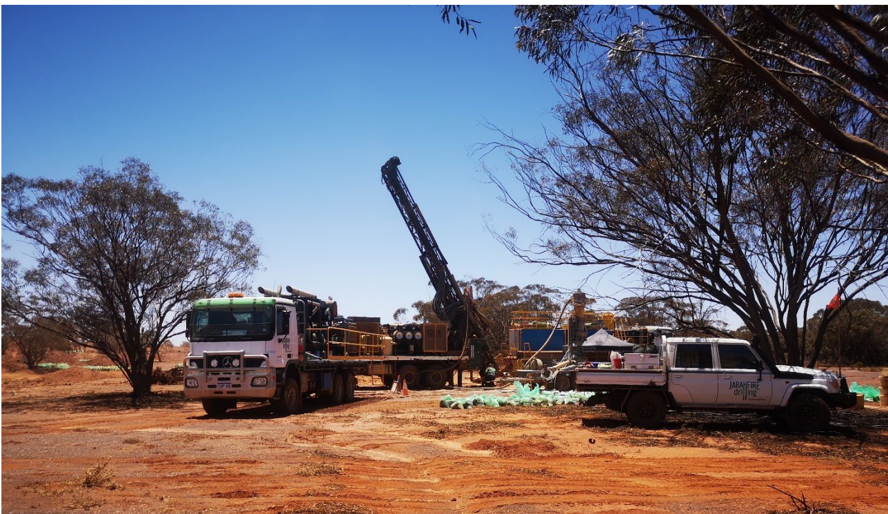
Figure 1: RC rig drilling Resource extensional holes at the Fingals Mining Centre (January 2022)
