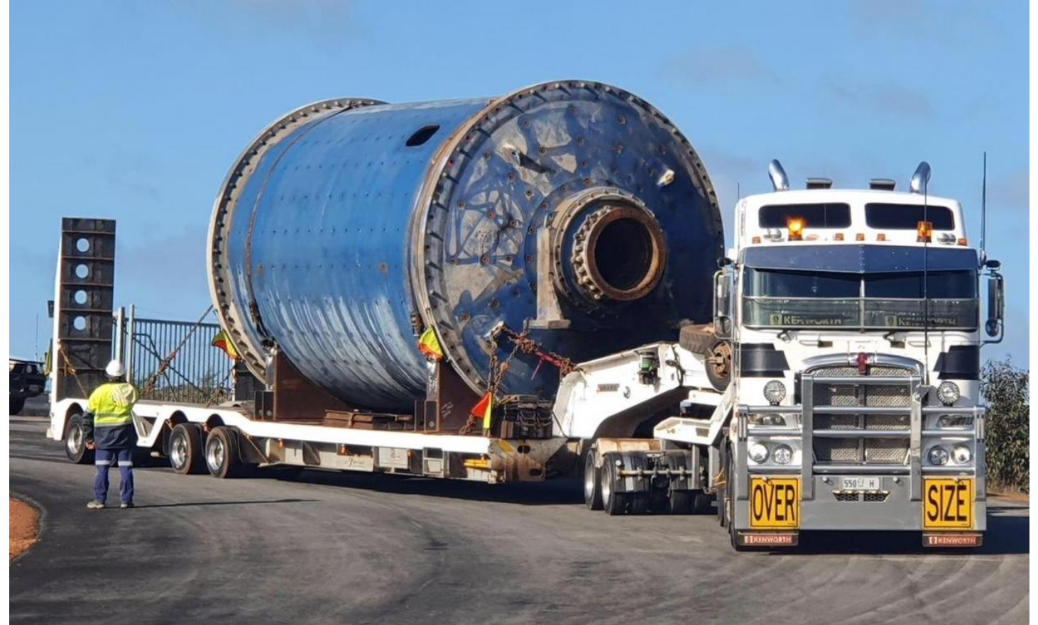
1.5Mtpa Outokumpu ball mills now in Kalgoorlie
