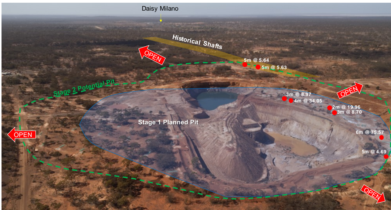
Figure 1. Aerial view of the Fingals Mining Centre looking south with high grade intercepts from recent drilling on the western side of the planned Stage 1 open pit.
