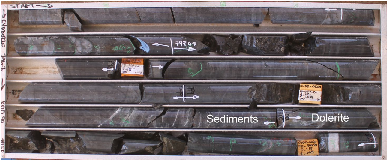
Figure 7: CYDD0220 drill core (796.2m to 800.99m) showing upper contact between sediments and poorly tested Coyote Dolerite. Note only one assay interval has been recorded for CYDD0220 at 0.40m @ 70.55g/t Au from 749.9m.
