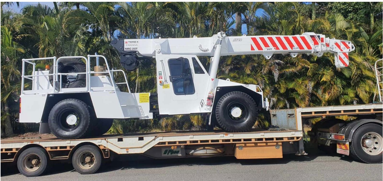
Figure 5: 20t Franna mobile crane being transported to site
