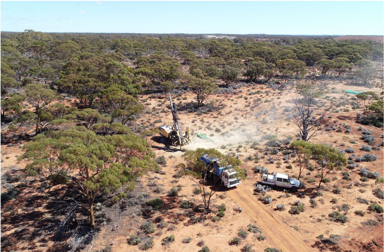
Figure 1: RC rig drilling Resource extensional holes at Jones Find North
