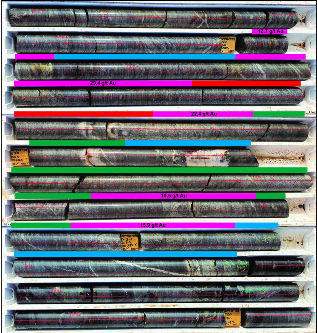
Figure 2: Annotated drill photographs of 6.45m @ 9.43 g/t Au from 228.51m (20MYDD002) with assay results (magenta >10 g/t, Red 5-10 g/t, green 1-5 g/t, blue <1 g/t). Note the intercept occurs close to the volcanic/sediment contact.
