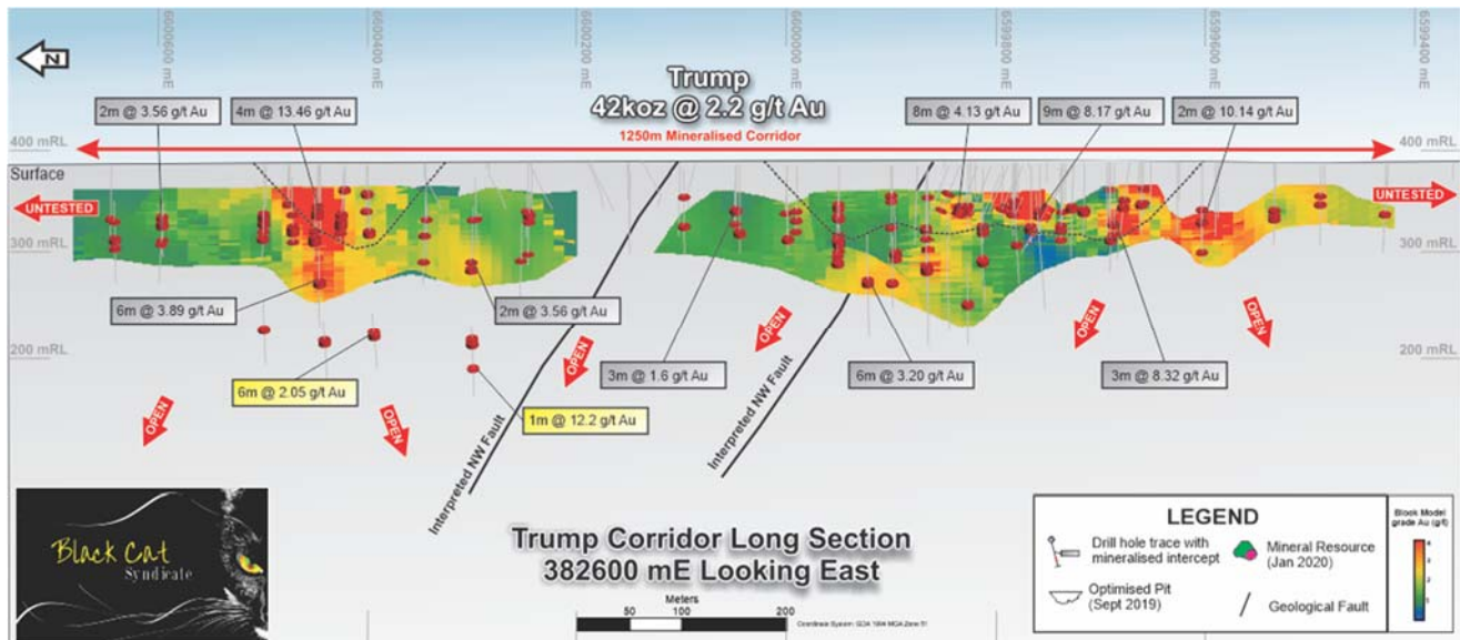
Figure 3: Longsection - Trump Resource (looking East at \geq 1 g/t Au) showing new drilling results.
