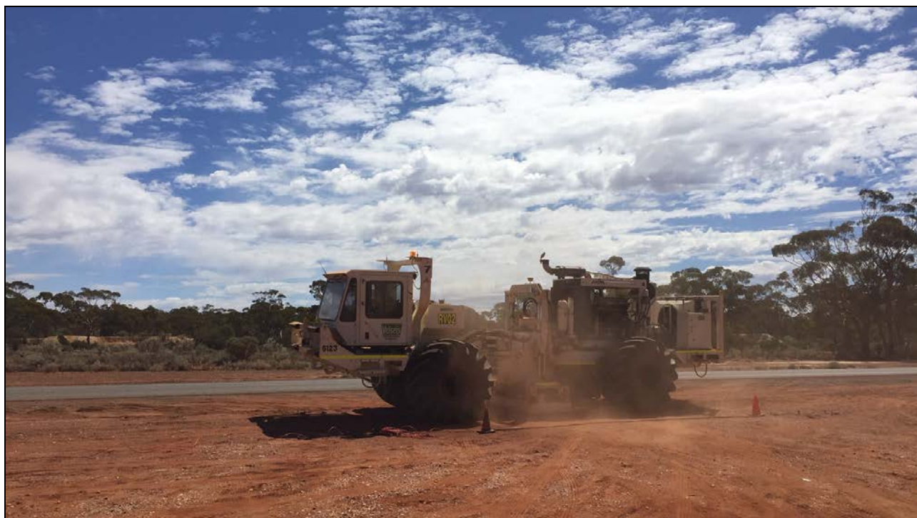
Figure 1: Renegade seismic vibrator currently in action in the Eastern Goldfields. These 80,000 lb units, operated by Velseis, are the most powerful seismic sources available in Australia and provide superior deep stratigraphic images.
