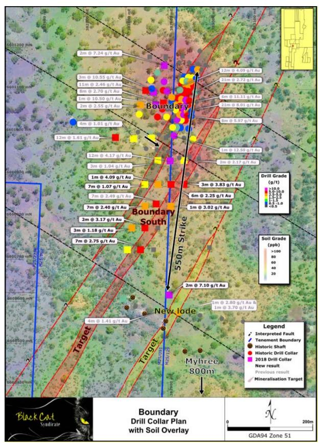
Figure 4: Drill collar plan at Boundary showing recent and previous RC drilling results and target zones.
