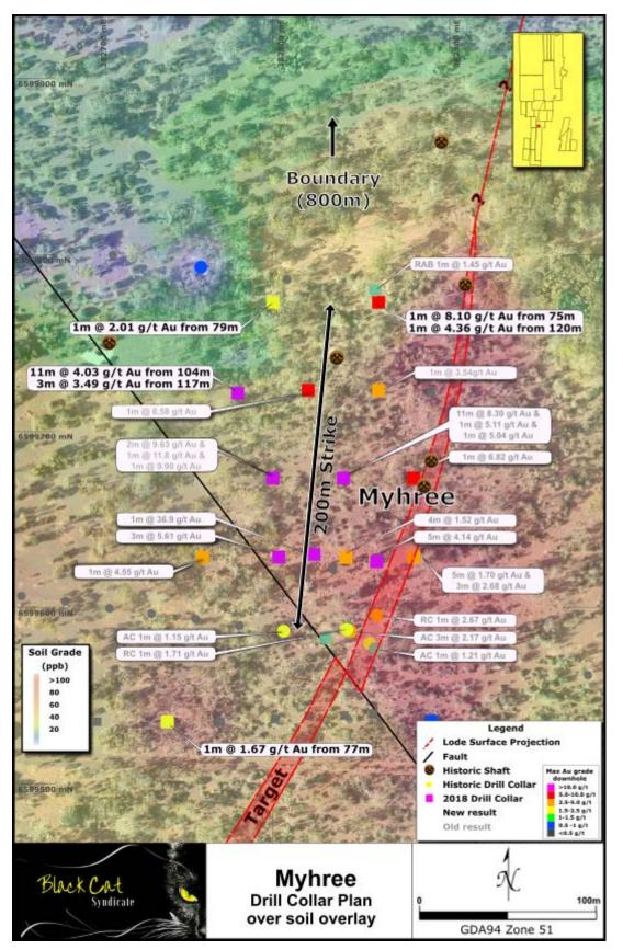
Figure 5: Drill collar plan at Myhree showing recent and previous RC drilling results.
