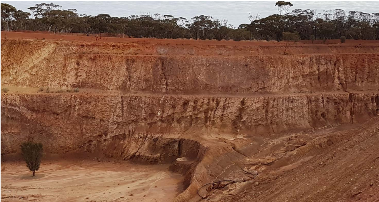
Figure 2: Photo looking at the north west wall of the Fingals Fortune open pit during the site visit. Low angle veining is clear within the pit walls.
