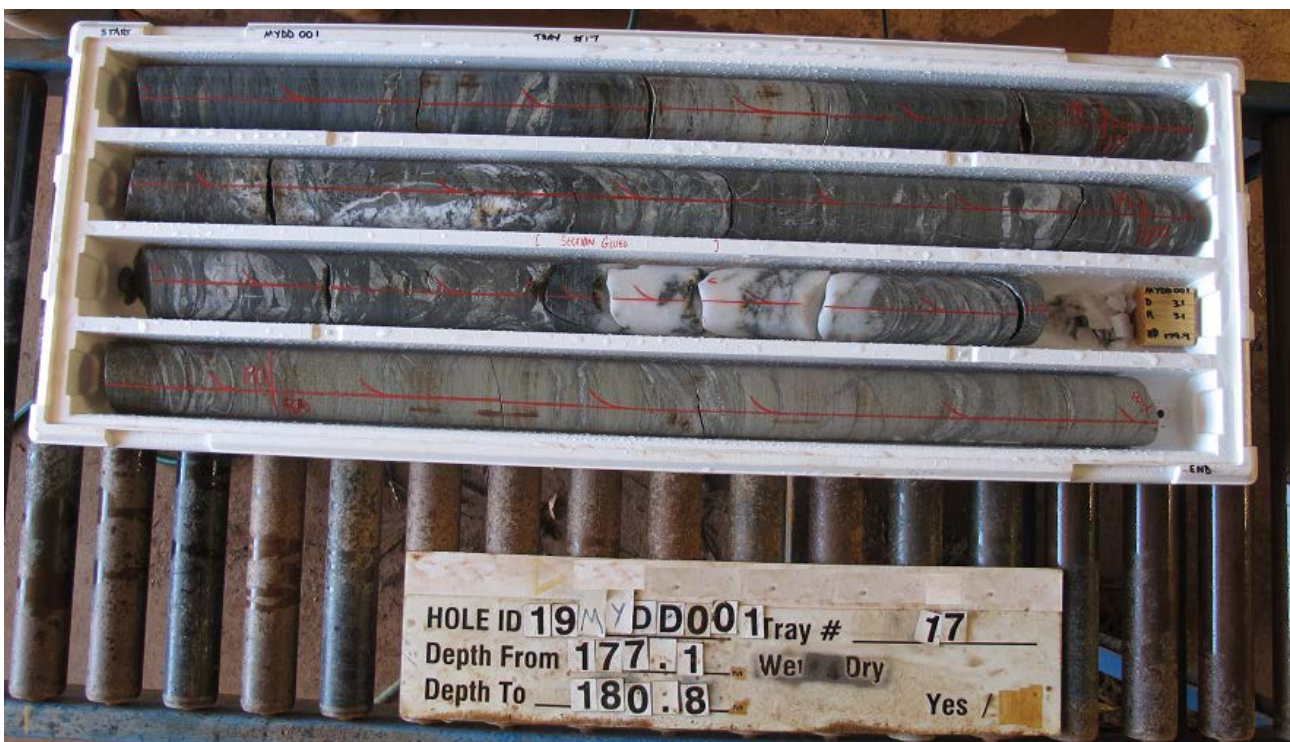
Figure 1. Oriented diamond core from hole MY19DD001 awaiting geotechnical logging.
