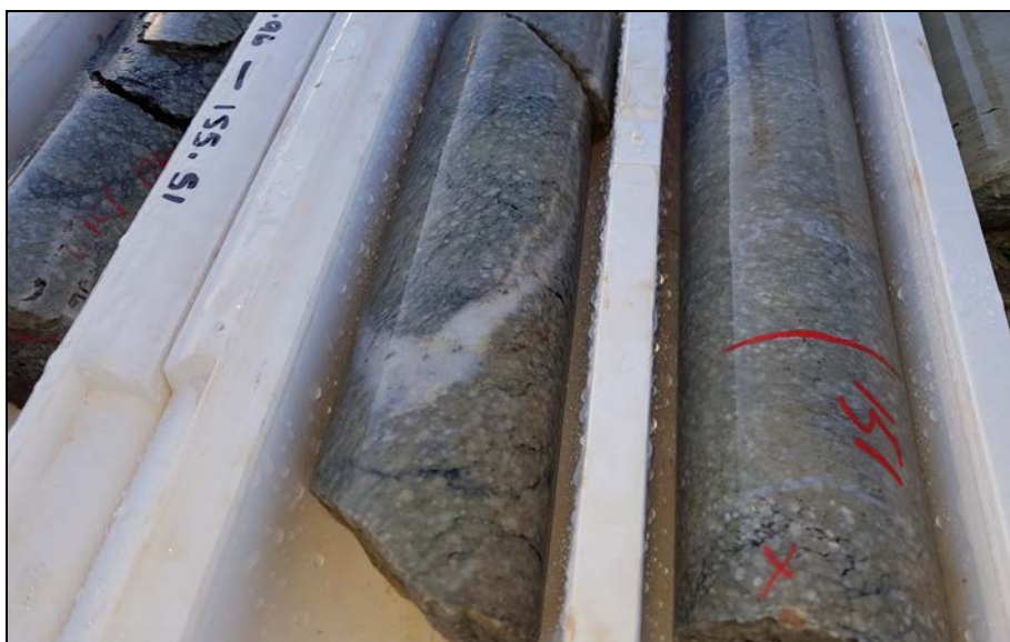
Figure 5: Porphyritic textured felsic host at Trump (18TRDD002)
