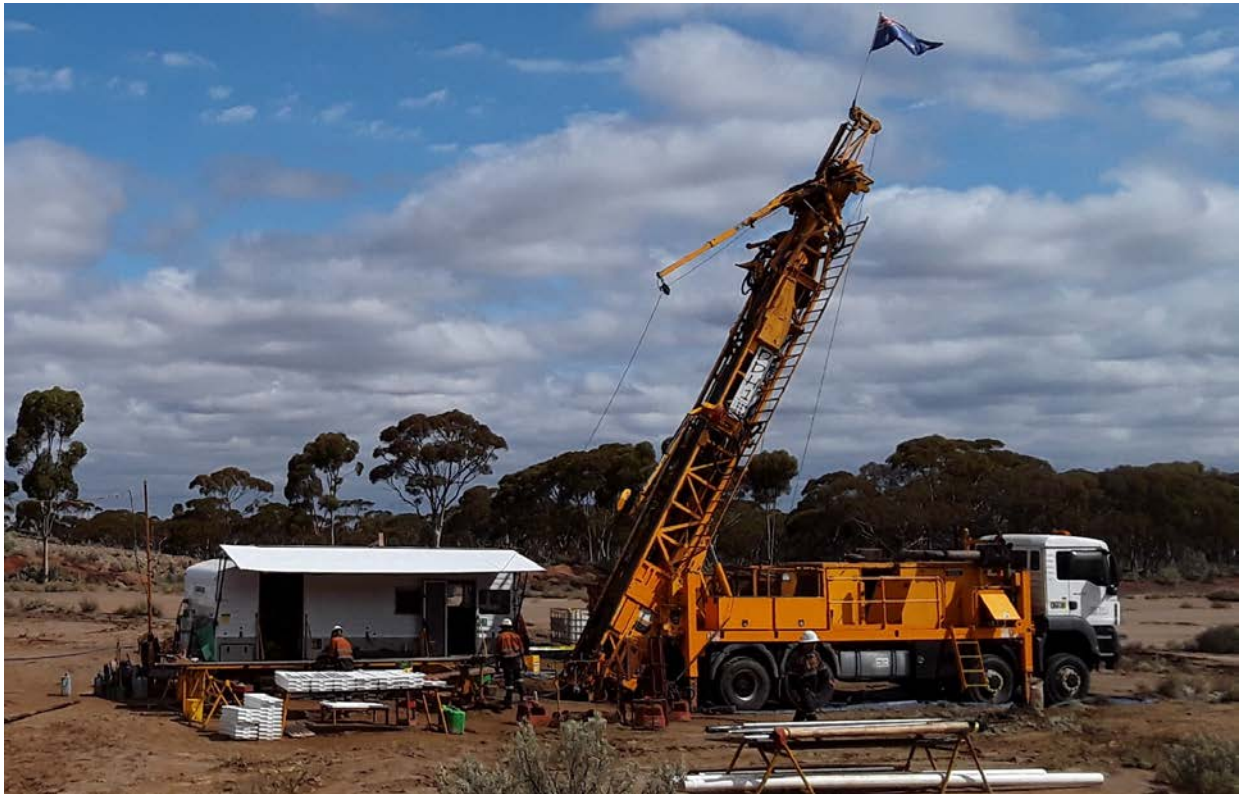
Figure 1: Diamond rig drilling at the Queen Margaret Mine, Bulong.
