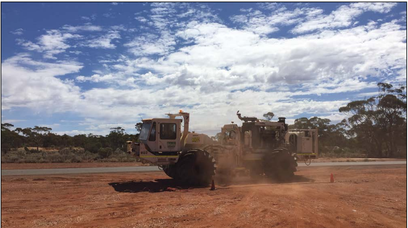
Figure 5: Renegade seismic vibrator currently in action in the Eastern Goldfields. These 80,000 lb units, operated by Velseis, are the most powerful seismic sources available in Australia and provide superior deep stratigraphic images.
