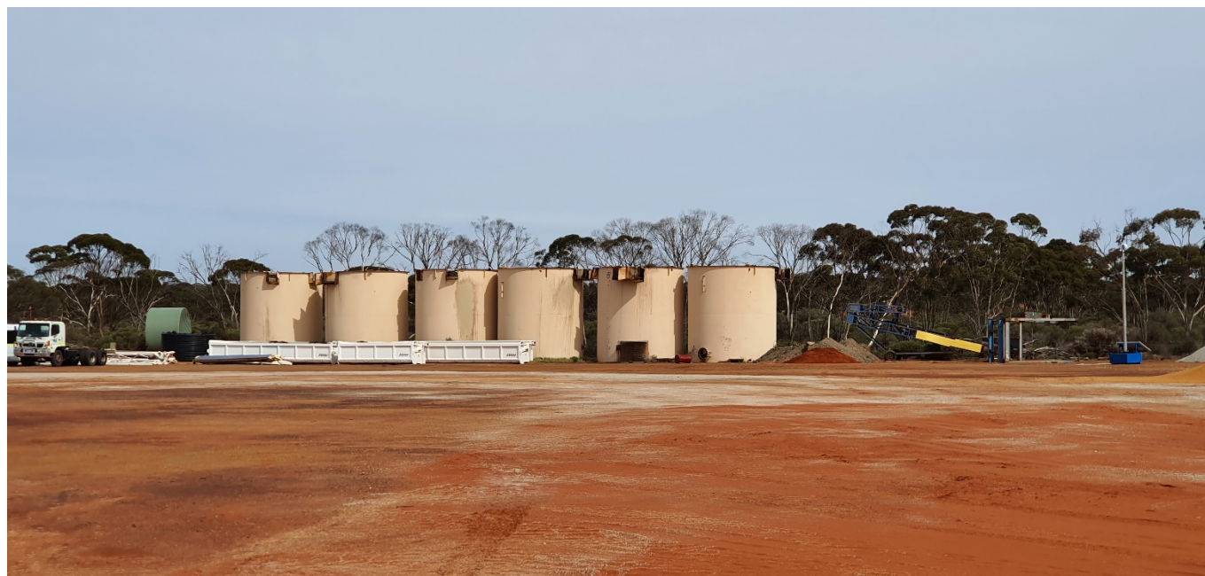
Figure 1: Black Cat’s Carbon-In-Leach adsorption tanks, located in Kalgoorlie, WA
